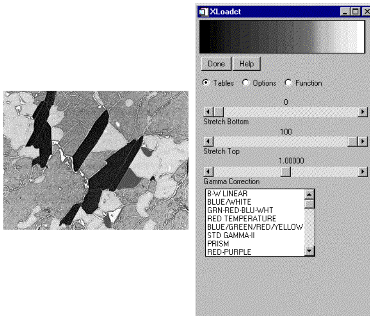
Figure 3-42: Resulting Image (left) and Color Table (right) of the Interactive Histogram Equalization in Direct Graphics
