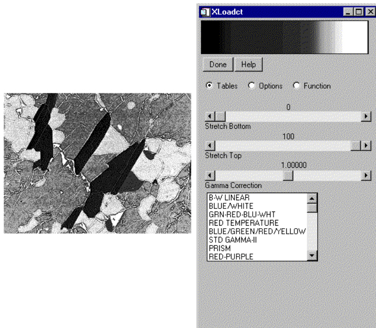
Figure 3-40: Resulting Image (left) and Color Table (right) of the Histogram Equalization in Direct Graphics
