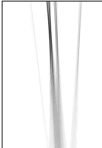
Figure 7-30: The Resulting Backprojection of the Scaled Hough Transform
