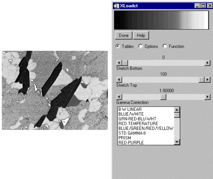
Figure 3-31: Resulting Image (left) and Color Table (right) of the Interactive Histogram Equalization in Direct Graphics
