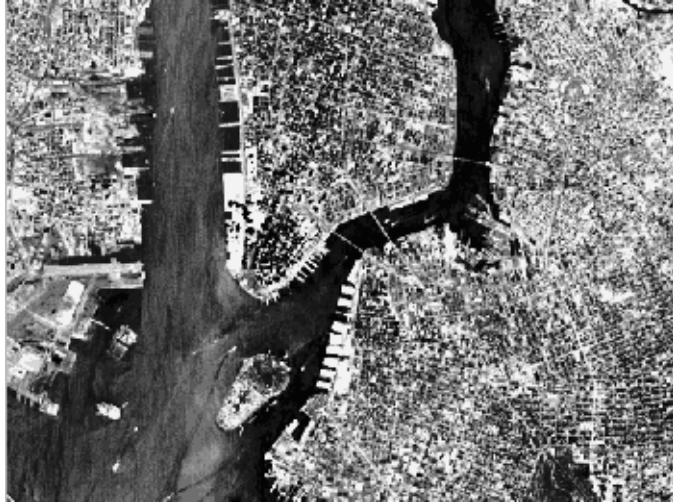
Figure 6-7: A histogram-equalized version of the image
